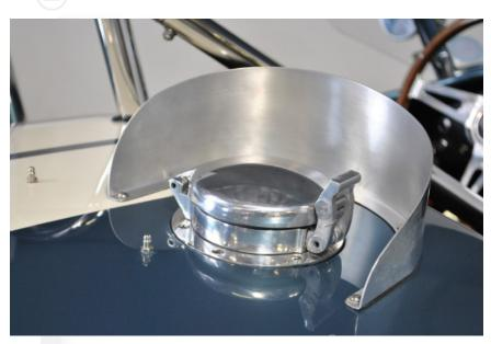
Optional Fuel cap diffusers can be fitted to FIA model cars.
