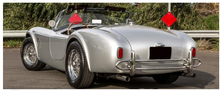
Slabside's feature straight cut fenders, where as the FIA features rolled fenders. FIA exhaust optional.
