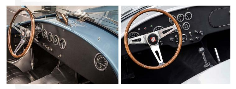
Slabside cars have the traditional roadster layout. FIA cars have two dash options, FIA and USSRC Spec.Aluminum interior is standard for FIA cars, where as carpeted surfaces are standard for Slabside cars. Glove boxes are standard for Slabside cars. (Leather seating shown optional)
