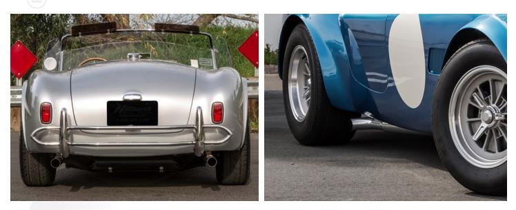
Sladside cars have under car exhaust, where as FIA cars have side exhaust standard.
